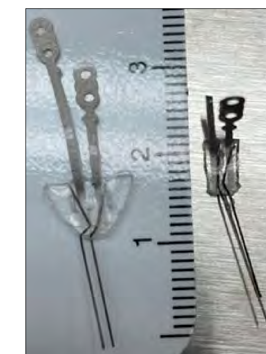
Figure 4. Final devices after curing and removal from mold before and after trimming. Trimmed device is 5mmx3mm and bottom nitinol wires will be cut to length during surgery.
